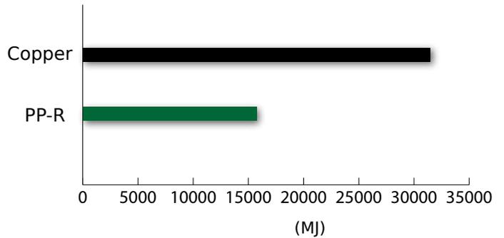
The study shows that a polypropylene piping system produces an average of less than 50% of the total emissions of a comparable copper piping system, as well as requiring less than 50% the energy to manufacture.
