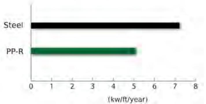
By reducing the amount of energy lost to friction in a piping system, the amount of electricity used by the pumps and motors can be significantly reduced. In the case of a steel hydronic system, 50% difference in the pipe friction factor can yield a 30% savings in annual energy use of the pumping system. The total percentage of the building’s energy use is dependent on the size and application of the system, as well as the other energy-consuming systems on the site.
