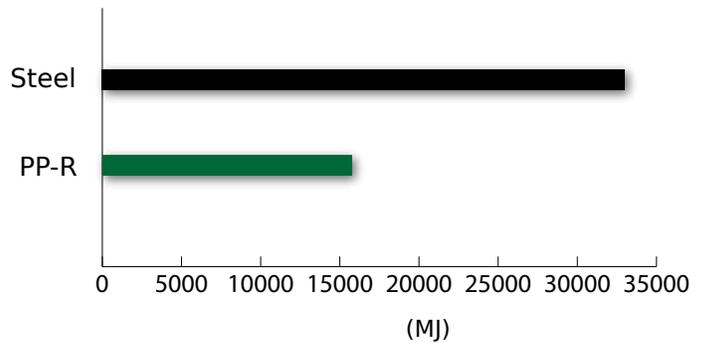
The study shows that a polypropylene piping system produces an average of less than 50% of the total emissions of a comparable steel piping system, as well as requiring less than 50% the energy to manufacture.
